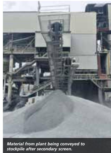
Material from plant being conveyed to stockpile after secondary screen.
