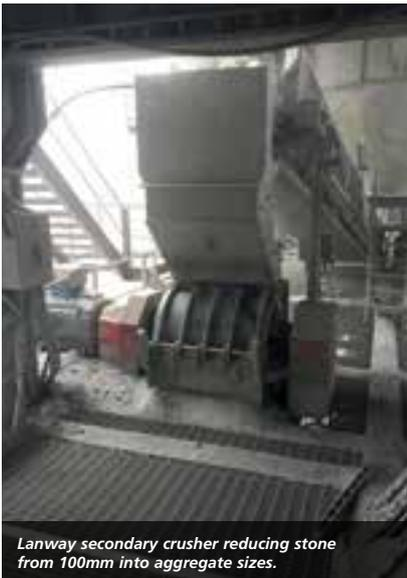
Lanway secondary crusher reducing stone from 100mm into aggregate sizes.
