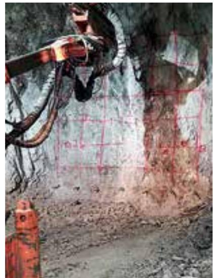
*A face which has been prepared and marked to the new standard, with the lower holes drilled first and plastic pipes inserted to ensure they stay 'open'.*
