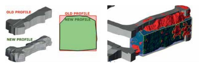
Figure 4: Comparison between Eagle and Deswik 3D As-Built solids for the same heading.
