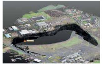
RGB Point cloud from eBee and greyscale intensity from TX8 Scanner combined data set.
