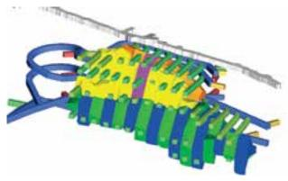
Figure 3: Long Term designs for stopes and development. One of the current active blocks.
