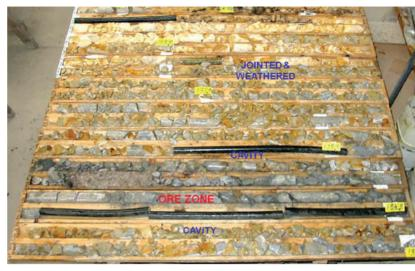
Diamond drill core showing weathered jointed ground
