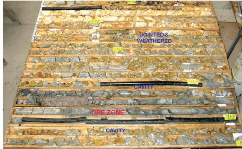
**Diamond drill core showing weathered jointed ground**
