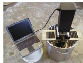
Figure n°1 – RHM 3000 ICAR Rheometer
