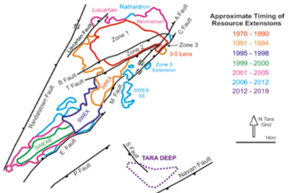
**Figure 1.** Plan of the Navan deposit showing the location and approximate timing of resource extensions, major faults and the location of the Tara Deep prospect. SWEX - Southwest Extension.
