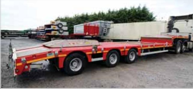
New 3 axle step frame low loader, extendable, with hook on aluminium loading ramps. 39ton payload, stake pockets and twistlock pockets.
