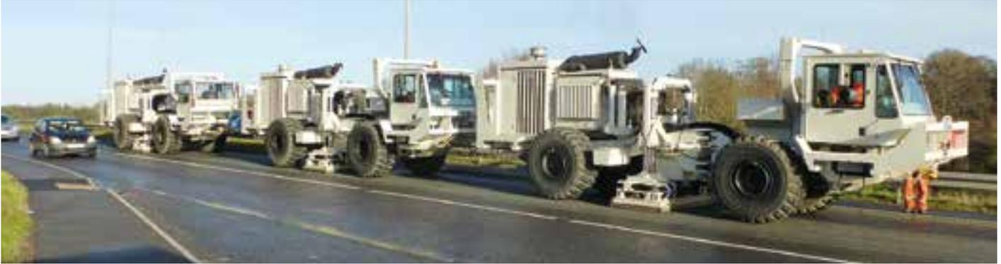
**Figure 2.** Vibroseis units working on a road in the Navan area.
