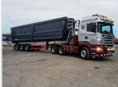
New Schmitz 80 cubic yard bulk scrap trailer, hardox steel body, barn doors with safety lock, front lift axle, very strong trailer with light tare weight, 8 tons , in stock ready to go
