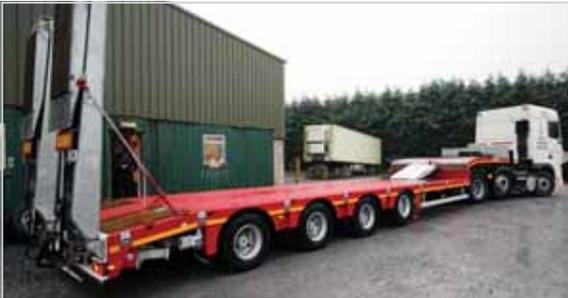
New Faymonville 4 axle step frame low loader, fixed bed, double flip ramps with hydraulic side shift, out riggers, marker boards, 48ton payload
