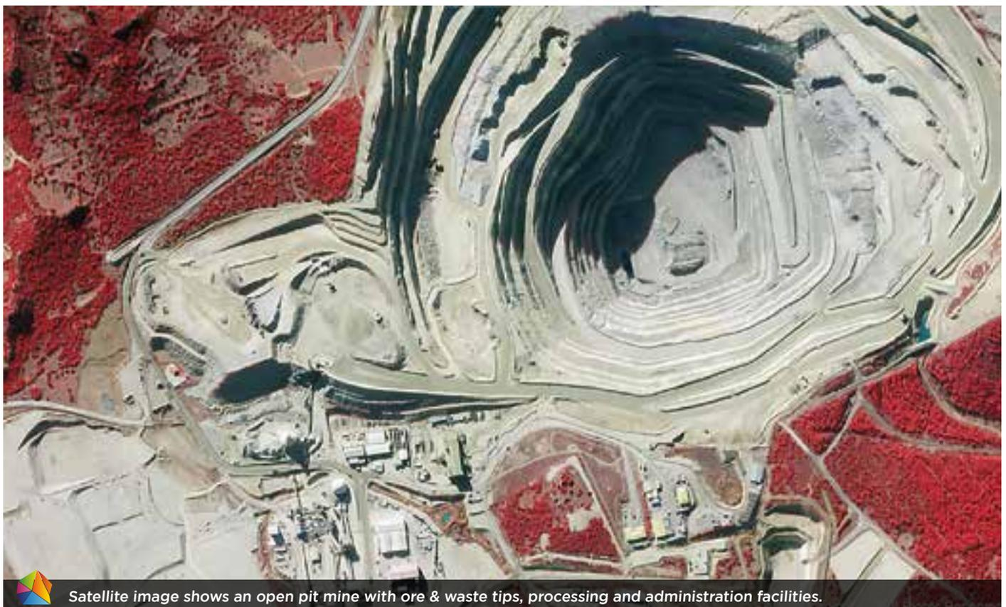
Satellite image shows an open pit mine with ore & waste tips, processing and administration facilities.
