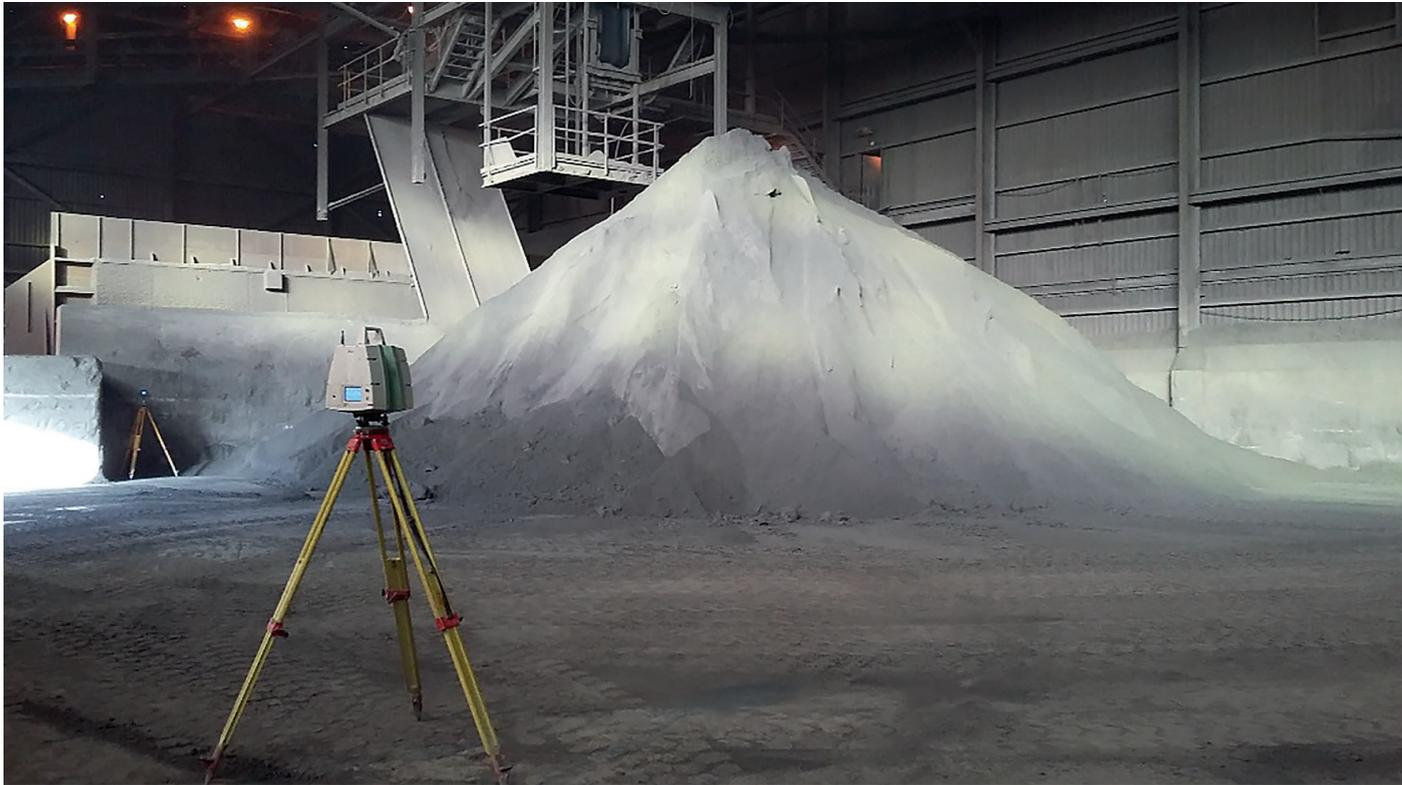
Figure 4: Laser scanning the Zinc concentrates stockpile for end of year accounting figures.
