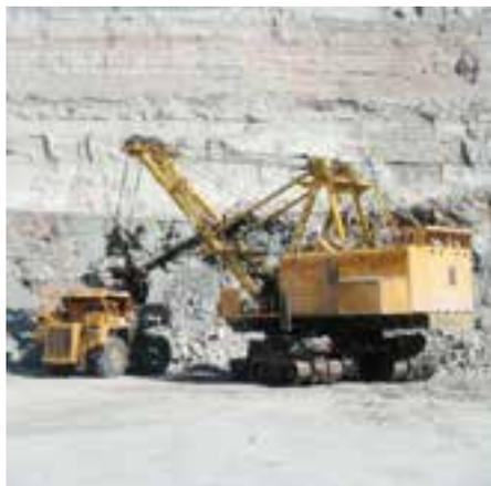
*Face shovel loading a 100t truck at an open pit diamond mine in Russia*
