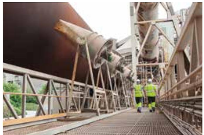
*Inspection of the kiln shell cooling fans, Platin Cement Factory.*
